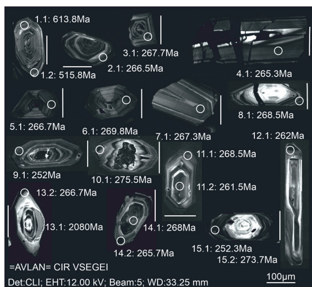
Fig. 5. Cathodoluminescence zircon images with indication of the age data (in Ma). The age data correspond to ^{238}\text{U}/^{206}\text{Pb} ages up to 1.0 Ga and to ^{206}\text{Pb}/^{207}\text{Pb} age data for >1.0 Ga.
