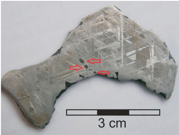
Fig. 10. Widmanstätten pattern in Smolenice. Three arrows show nodules of troilite (photo: S. Antalík).
