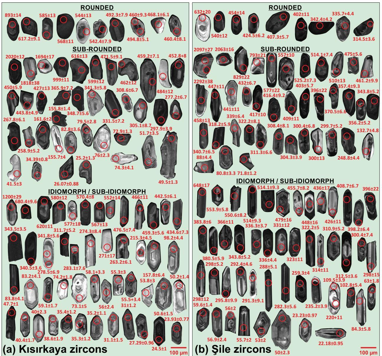
Fig. 5. Zircon cathodoluminescent images for the Kısırkaya (a), and Şile (b) sands. Red circles represent the dating points.
